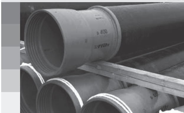
井戸管 Well pipes
