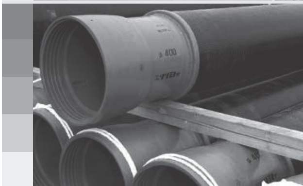
井戸管 Well pipes
